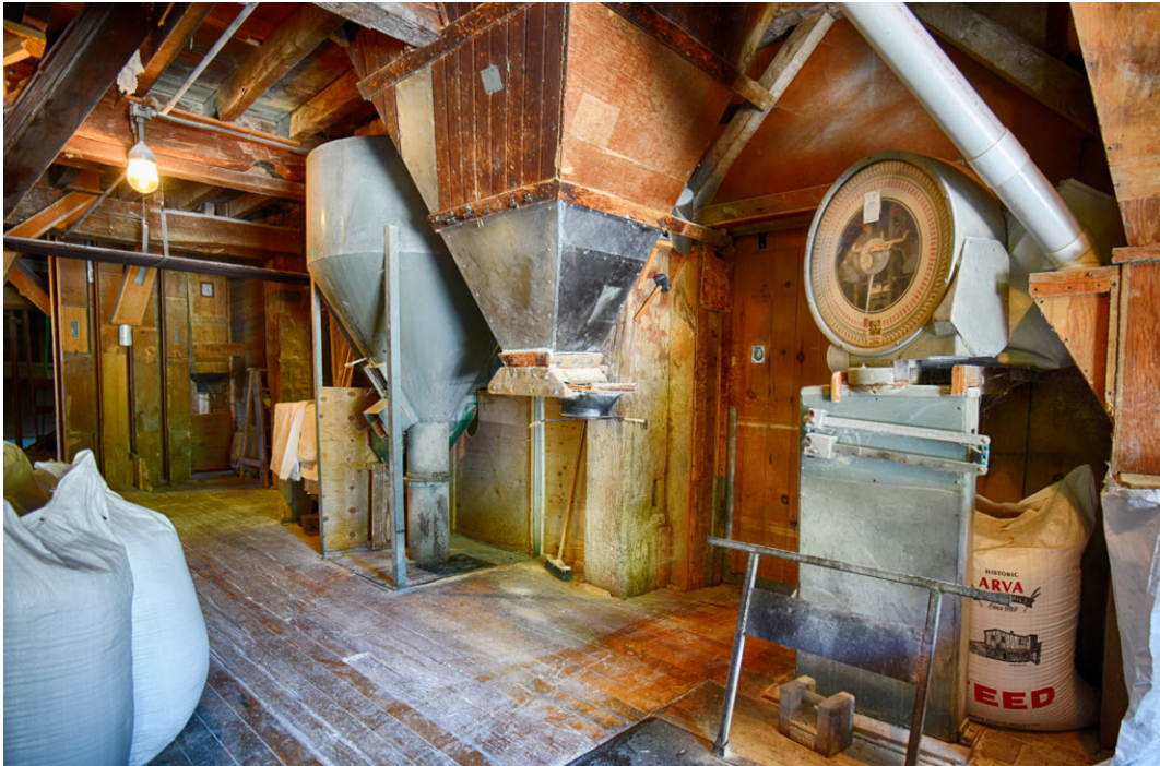
Scale used to weigh the various components of feed and the finished by-products of milling. (Photograph courtesy of Joe O’Neil.)
