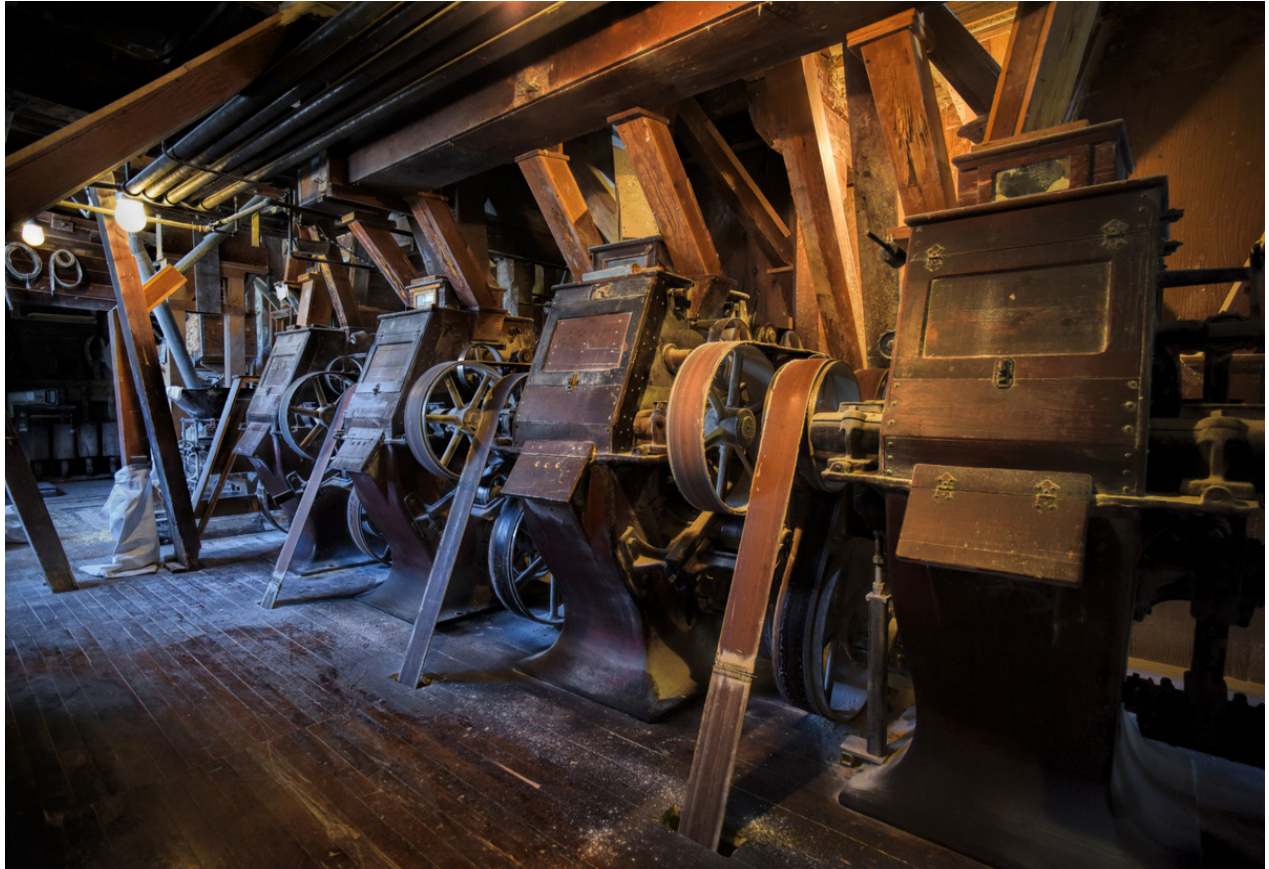
Roller bins in the Arva Mill used to ground wheat kernels into flour.
