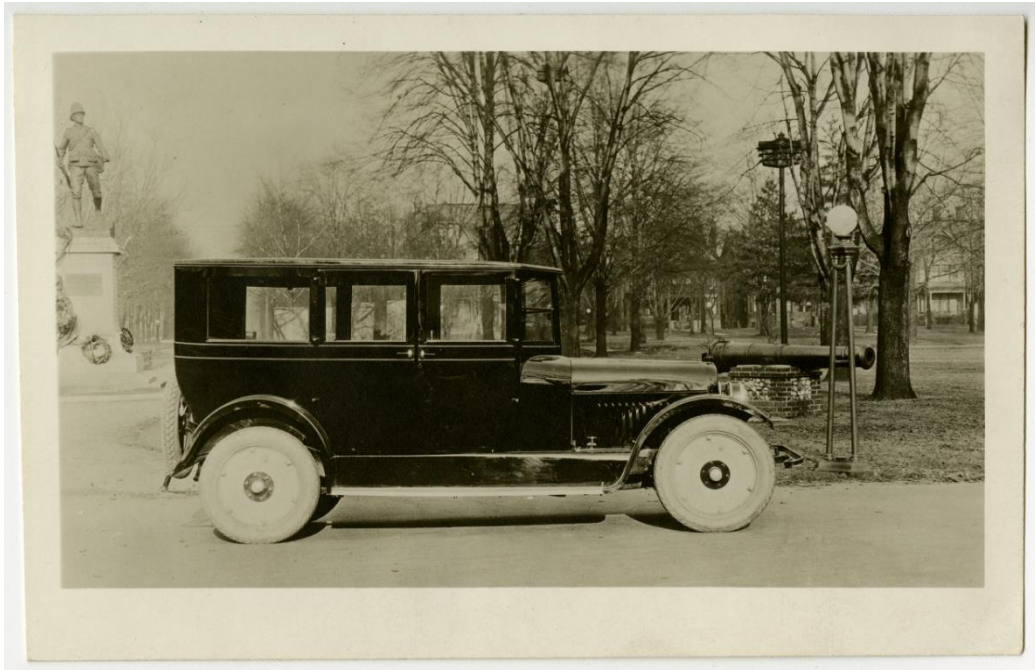
A "London Six" pictured in Victoria Park, 1922. Note the distinctive wooden disc wheels designed to reduce noise and tire wear. Photo Source: Western University Archives, London Motors and Stansell Family Fonds
